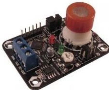
Gambar 2. Sensor gas MQ-3
