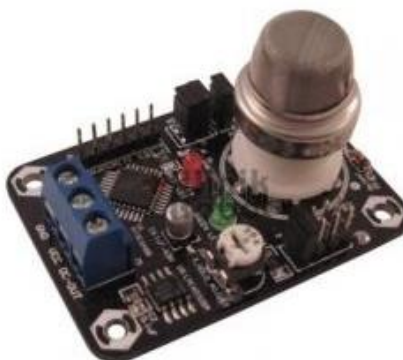
Gambar 3. Sensor Gas MQ-4
