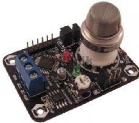
Gambar 1. Sensor Gas MQ-135
