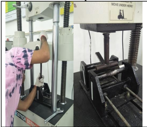
Gambar 3.5 Proses Uji Bending
