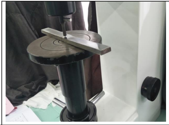
Gambar 3.6 Proses Uji Rock Well
