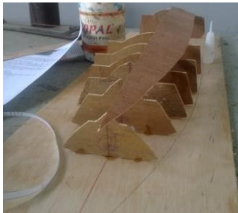
Gambar 4. Proses Pemasangan Station
