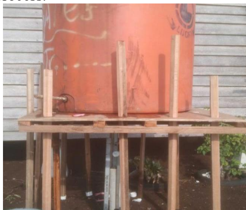
Fig. 1 Testing Models of Mini Pile Settlements
