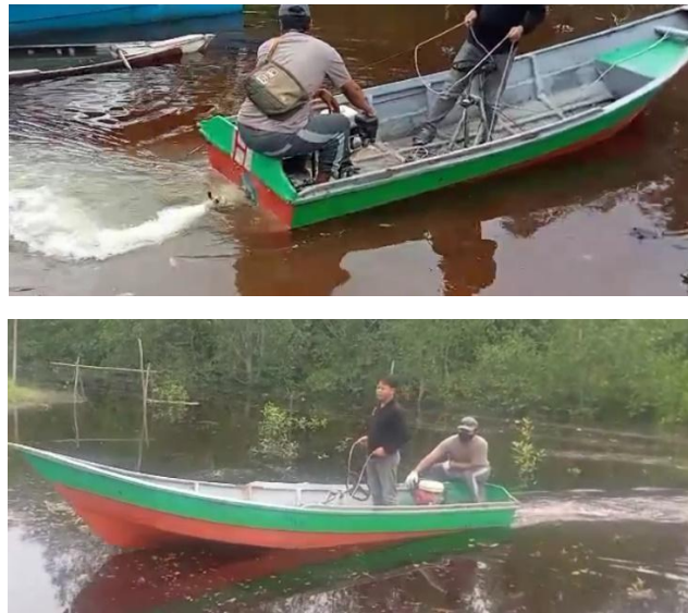
Figure 9. Water Jet Testing on a 1 GT Boat
